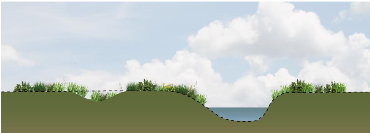
Figure 4.3 Indicative cross section illustrating floodplain scrapes.
