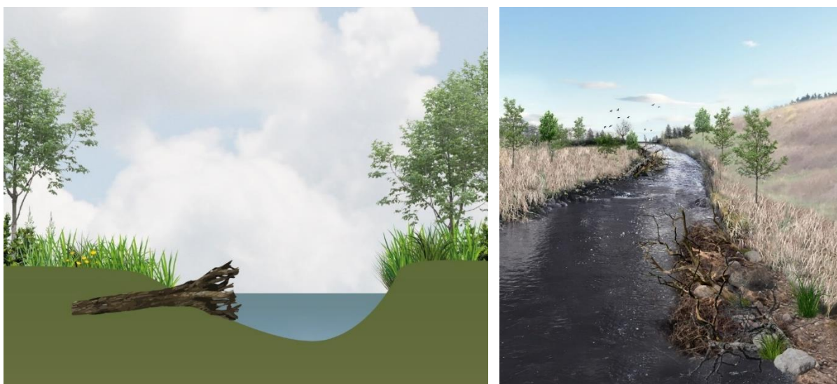
Figure 4.8 Illustrative example of large wood placement. Left: cross-sectional view of a channel, Right: structures installed on alternate banks.
